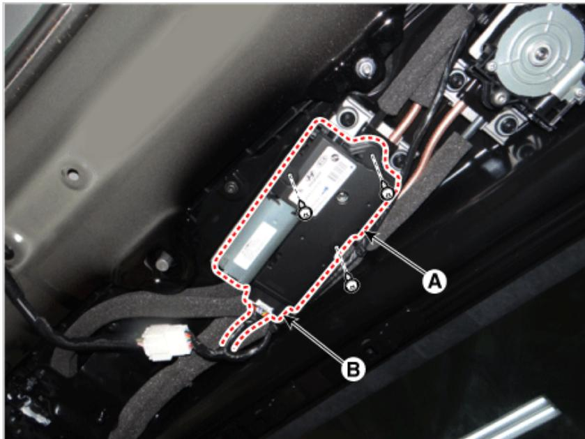
4. Remove the roller blind motor (A) after loosening the screws and disconnecting the connector.
